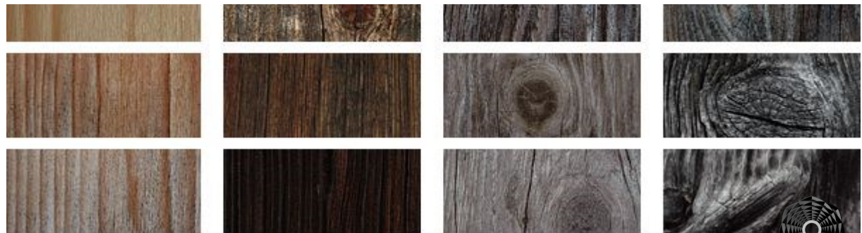
Changes in the wood structure due to direct weathering and leaching of the natural "wood glue" lignin
